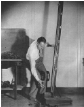
The drop test was used to determine how strong a phone needs to be.
